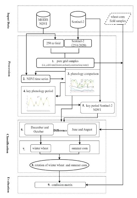
Fig. 2. Workflow of key phenological stage difference index method.
